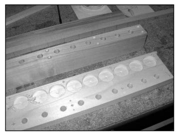
Figure 14. Unfinished pouch board and toe board.
