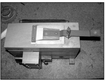
Figure 11. Top view of tremulant showing hinged weighted arm.
