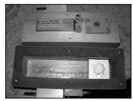
Figure 10. Center and bottom layer of tremulant.
